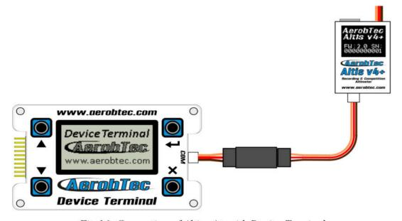
Fig 16: Connection of Altis v4+ with Device Terminal
