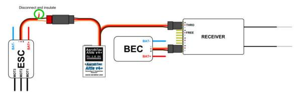
Fig 4: Connection of Altis v4+ with external BEC
