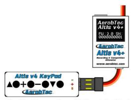
Fig 15: Connection of Altis v4 KeyPad
