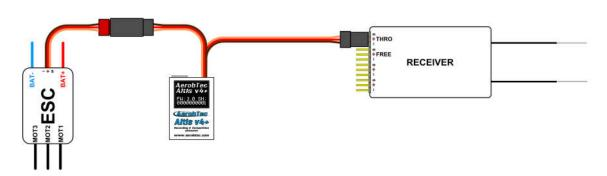
Fig 3: Connection scheme for competition use (ESC - electronic speed controller, THRO - throttle receiver channel)
