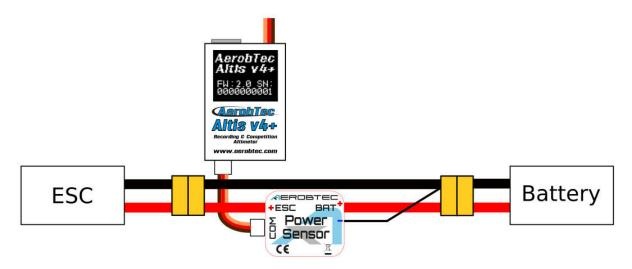
Fig 18: Power sensor connection
