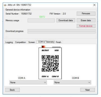
Fig 12: COM A / COM B Telemetry, Keypad or Live output settings
